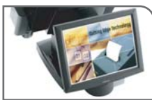
LM-6501 / 6101 Integrated secondary 15"(LM-6501) / 12.1" (LM-6101) TFT LCD display for advertisement and promotion on rear lower base
