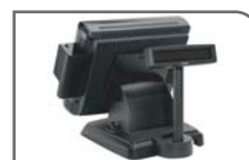
PD-2602 9 mm 2 x 20 VFD display, 5X7 dot matrix, default RS232 interface, optional USB interface
