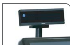
PD-2501 11 mm 2 x 20 VFD display, 5X7 dot matrix, RS232 interface
